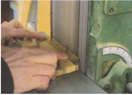
▲ Pic 5 Held together by rods, this was placed on the jig, and the metal was sanded back to the handles
